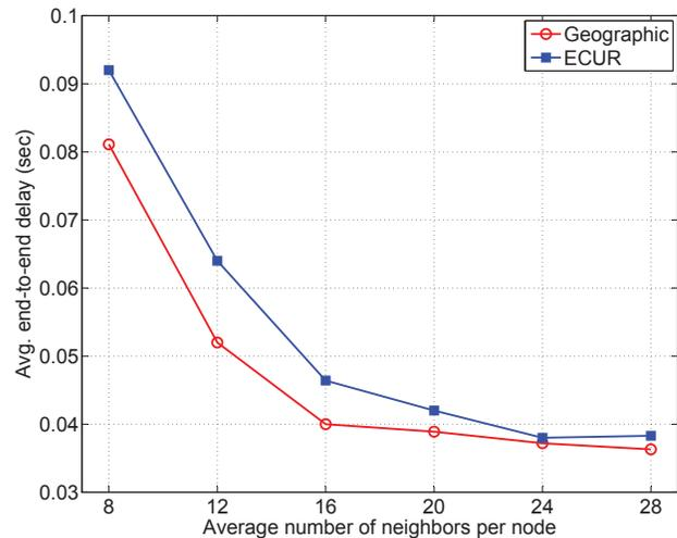
Fig. 3: Average end-to-end delay under different network density.
