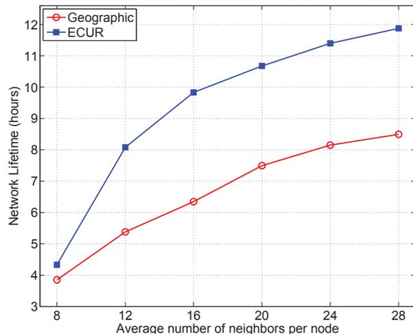
Fig. 2: Network lifetime under different network density.
