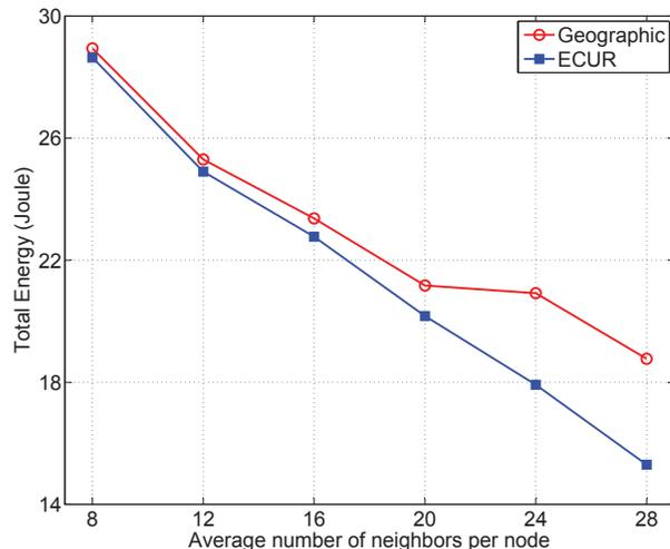
Fig. 1: Total energy consumption under different network density.
