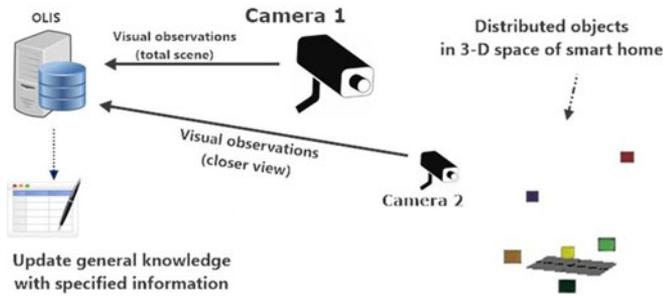
Fig. 1. Observing distributed objects with two far and close cameras.
