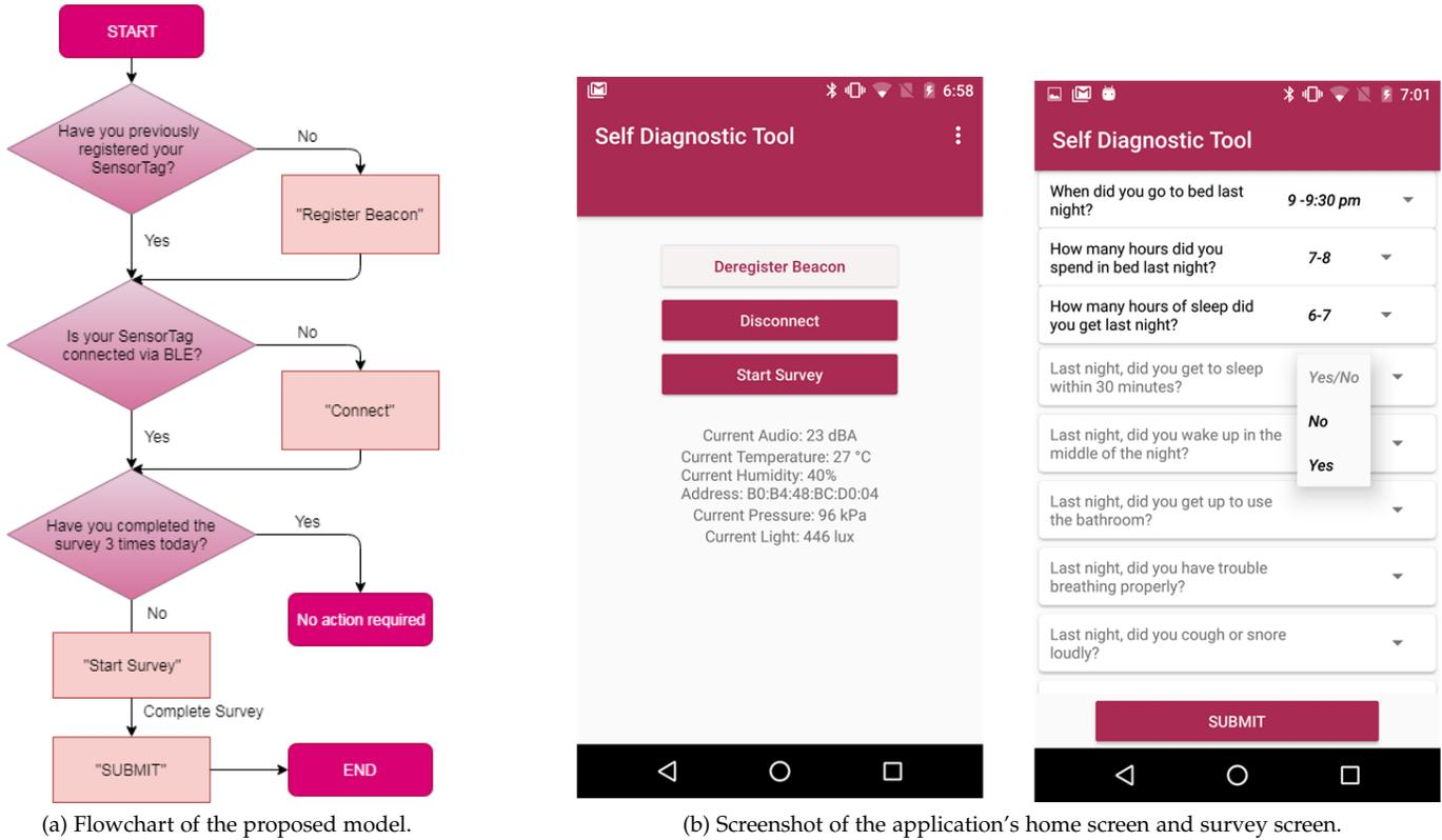
Fig. 2: Flow chart for the mobile application (2a) and screenshots of the application's two main screens (2b).
