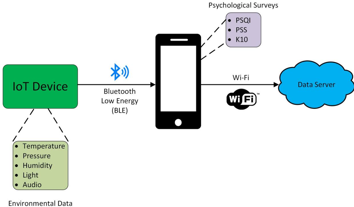
Fig. 1: Flowchart of the full framework, including the IoT device, the mobile application, and the server.
