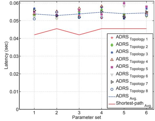
Fig. 3: Average packet latency for the parameter sets of Table I.
