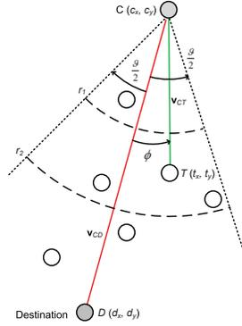
Fig. 1: Selection of a forwarding candidate set for the current node  $C$  towards the destination  $D$ . A neighbor node  $T$  is in the set if it is in distance larger than  $r_1$  and its inclination angle  $\phi$  is smaller than  $\pm \frac{\theta}{2}$ .
