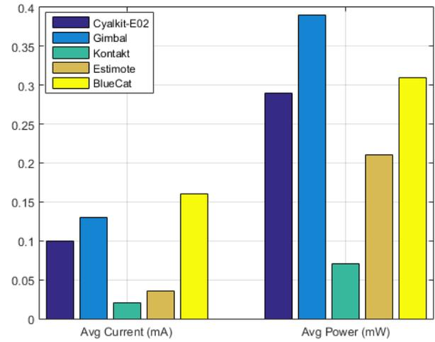
Fig. 2. Current and Power characteristics of beacons.
