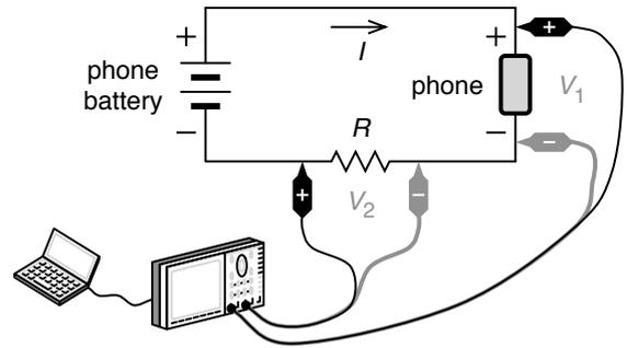
Figure 2: Setup for measuring the power supplied by the battery to the smartphone.
