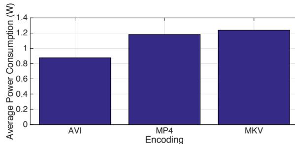
Figure 6: Average power consumption of videos with different encoding on MEGA.
