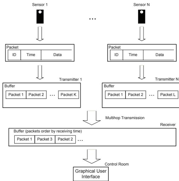
Fig. 2: Forming packets and transmitting
