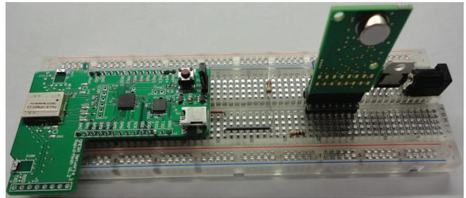
Fig. 1: Temperature Monitoring Board
