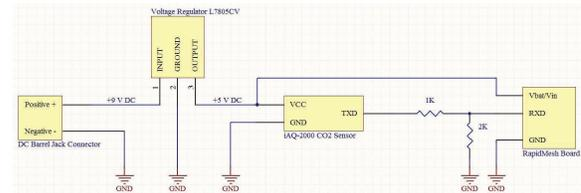
Fig. 3: Circuit schematic
